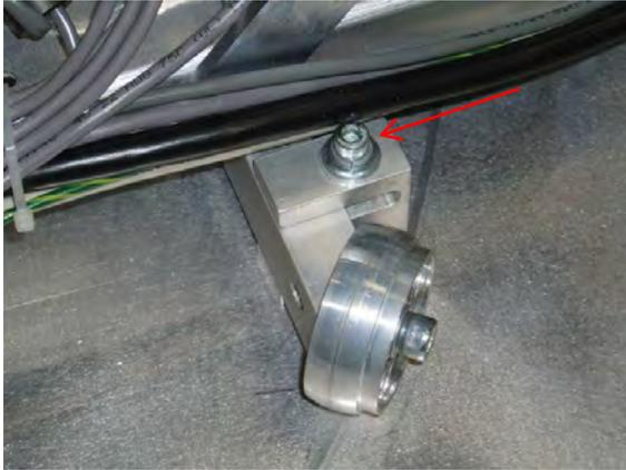
3. The back Power Panel has been placed in a "Shipping" position to secure during shipping. This needs to be adjusted to its operational position. Remove the top 2 screws. The remaining 2 mounting screws are stored below the panel.
