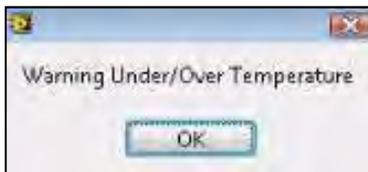
**Temperature Monitoring Failures:** The system is designed to send a Failure message to the user if the internal temperature of the machine is 20° C or lower OR 60° C or higher. This Failure message would display in the “CB Scanning Device” Acquisition software at Startup and just before a scan is captured. If this condition occurs the error message will force the acquisition program to terminate and disallow any scanning.
