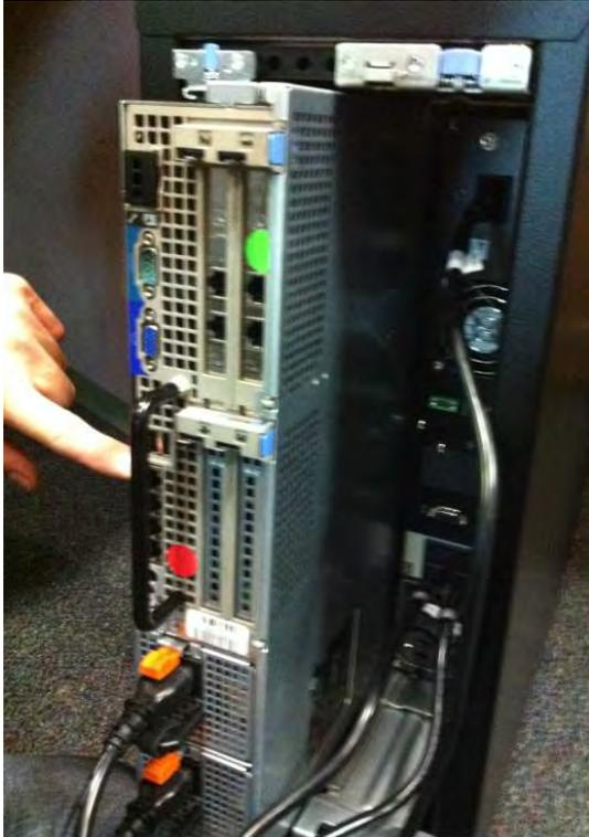
Turn ON the server and verify that all VM's are powered ON. You must remove the right hand side cover to access the ON button to the server.
