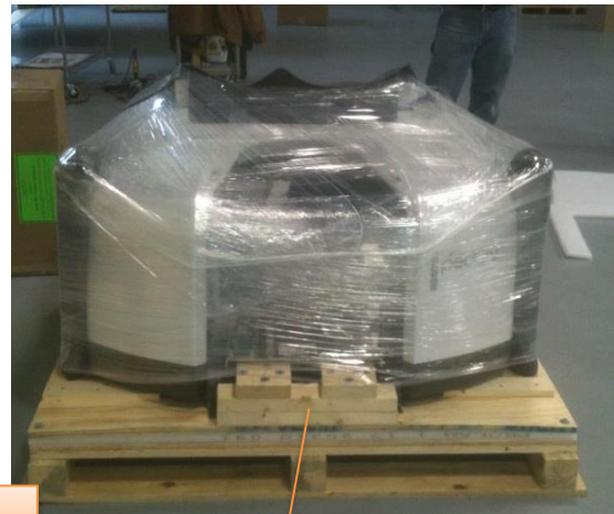
Machine shipping mount/bolts.
