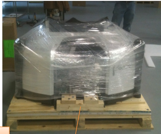
Machine shipping mount/bolts.
