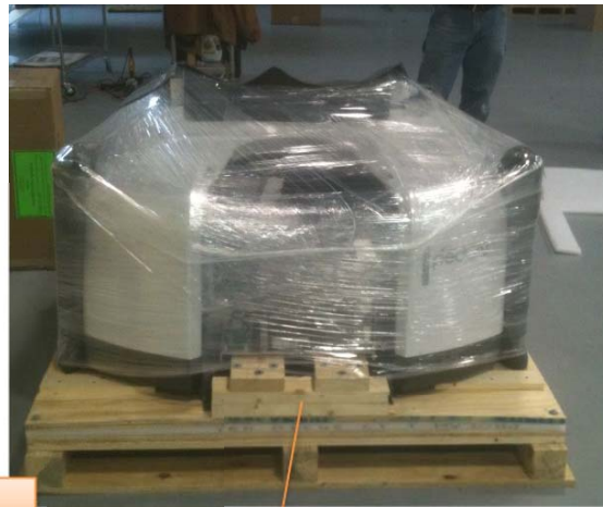
Machine shipping mount/bolts.
