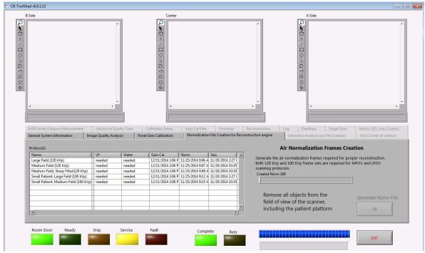
This calibration will create a norm file for each of the protocols listed. In order to do this, a scan must be taken using each protocol. **Ensure that there is nothing in the FOV, including the patient platform.** To start, click on the first protocol in the list, which will appears as follows:
