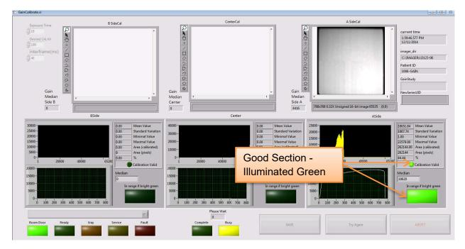
If the section was successful, there will be 2 green lights illuminated under the calibration side that was completed to show a successful 1/3 of the Panel Gain Calibration. Both the Calibration Valid and "In range if bright green" will illuminate bright green for a successful portion of the gain calibration as shown in the above picture. If the section was not successful, the lights will remain unilluminated.
