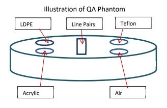
1. Place the QA Phantom on the devices patient platform using the circular positioning guides to center it on the platform.
