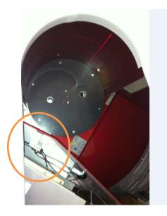
Horizontal Laser Lights: The lower light should be 10 cm above the platform. The upper laser light should be 20 cm above the platform. If not, adjust each adjustment screw on the horizontal laser light mechanisms to achieve proper location.
