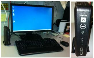
Connect the Viewing Station/MD Thin Client Terminal to the server. Plug in the Thin Client Terminal box, Monitor and mouse. Turn the Thin Client Terminal box ON.
