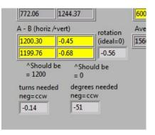
The adjustments are shown both in turns needed and degrees. Use the format that is most comfortable. If adjustments are needed, adjust the screws on the mounting plate for the panel as shown below:
