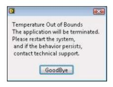
*Startup:* Note that there is an Internal Temperature gage in the Startup Screen. If in the Startup Screen and the temperature monitor has detected temperature out of range, the failure message will display during the Startup sequence.
