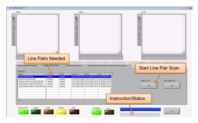
On this tab the Line Pair and Water QA scan dates are shown. In the image above, all of the Line Pair (LP) and Water QA scans still need to be done.
