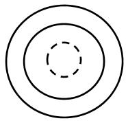
The most <u>outer circle</u> is for the <u>Full, both feet procedure option (35 cm diameter)</u>. This is for a scan that needs to include both feet. Both feet should be positioned within this circle in order to capture both.
