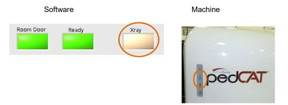
3. When the audible buzzer and "X-ray on" light turn off, it is OK to release the exposure switch.
