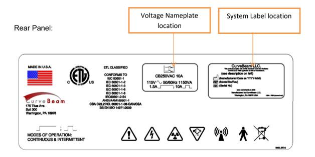
Voltage Nameplate for opening in Rear Connector Panel and Rear Panel:
