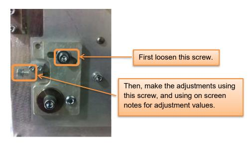
If the adjustments are needed, once made, rerun this calibration.
