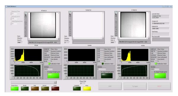
The B SideCal will now also show if the Calibration was valid or not, by illuminating the green lights for success and not illuminating them for failure. The lights for success or failure are same for all three calibration sections.
