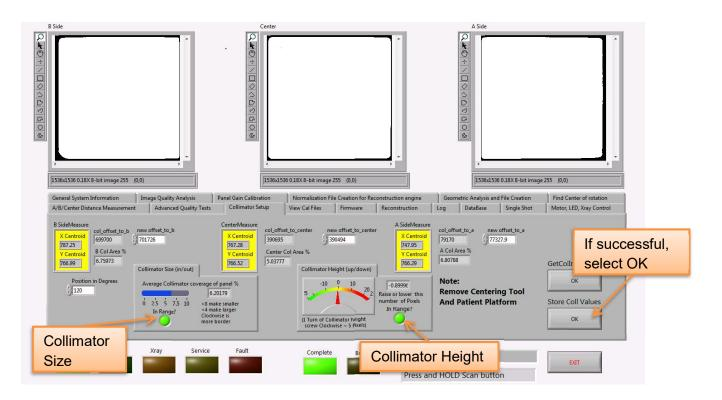
Successful completion is two green lights, one in the Collimator Size and one in the Collimator Height boxes. If both lights are green, select the StoreColValues OK button.
