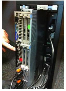
Turn ON the server and verify that all VM's are powered ON. You must remove the right hand side cover to access the ON button to the server.
