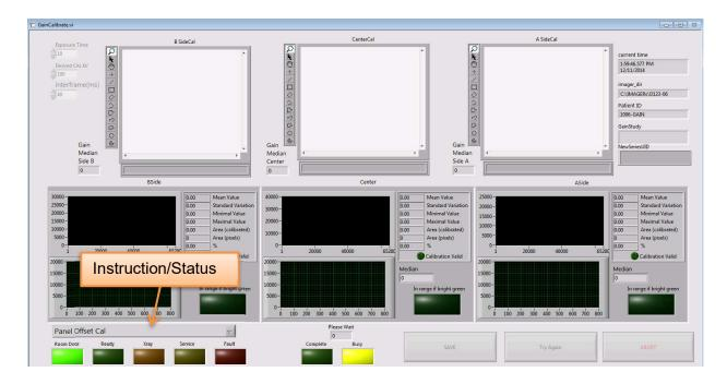
The user will receive messages and updates on what is happening as well as instructions on what to do (when to fire x-ray) in the window on the lower left corner. There will be a message to fire x-ray to perform the gain calibration on A Side. When prompted, Press and Hold the Scan button to fire the x-ray.
