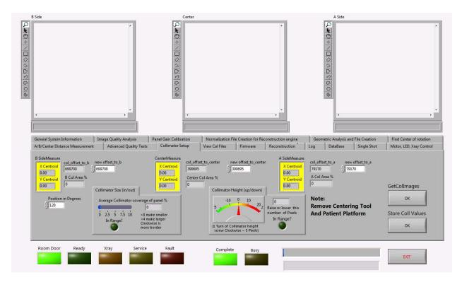
Click on the GetCollmages OK button to start the calibration. This will start the calibration and instructions will appear that will include instructions to fire the x-ray. When prompted, Press and Hold the Scan button to fire the x-ray. X-ray will be fired **THREE** times.
