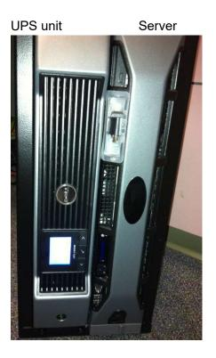
Remove the left cover from the bottom clip. Connect the battery plug. Turn the UPS ON with the button below the plug and verify that it is powered. Replace the cover.
