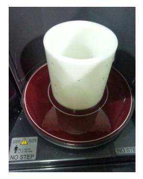
The Geometric Calibration will need to be run on both a MFOV and a LFOV scan, but only one of each. For the purposes of viewing the BB's better, the 120 kVp scans should be used. This procedure will be run first using the Large Field (120 kVp) scan and then again using the Medium Field (120 kVp) scan.
