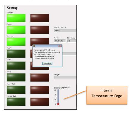
*Scan:* If in the Procedure Tab and the temperature monitor has detected temperature out of range, the failure message will display once the OK button is clicked.
