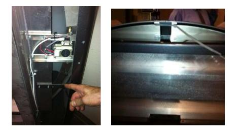
Then the 4 Gantry Clamp Shipping screws can now be removed. These secure the gantry during shipment. They are at the base of the gantry.
