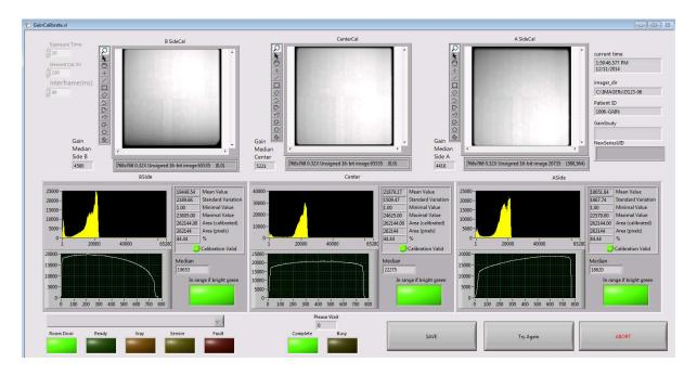
As for the A and B sides, the two green lights indicate success for the Center Cal, unilluminated lights indicate failure. In the image above, all three sections have passed successfully.
