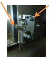
8. <u>Mount the X-Ray tube head:</u> There is only one twist lock connector and 4 screws for mounting.
