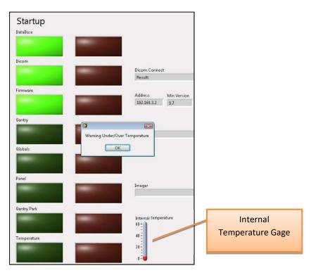
*Scan:* If in the Procedure Tab and the temperature monitor has detected temperature out of range, the warning message will display once the OK button is clicked.
