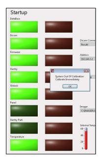
*Scan:* When the monthly calibration and checks are due, the message will display in the Procedure Tab when the OK button is clicked. When the message displays, the user should click OK and then should contact CurveBeam technical support who will assist in the calibration and checks via remote access. This message will repeat at Scan time until the procedures are completed. Once the procedures are completed the warning message will be reset by CurveBeam technical support.
