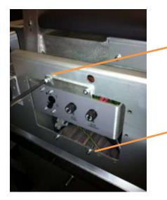
Shipping position of back Power Panel. Remove these 2 top screws
