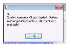
Select OK. Perform the remainder of the Line Pair scans. If the protocol has "needed" listed under the LP column, then that protocol still needs a LP scan. Once all of the entries in the LP column are filled in with date and times and no longer say "needed", remove the Line Pair Phantom from the scanner.
