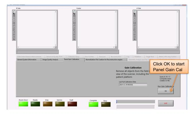
Before starting the Panel Gain Calibration, **ensure all objects are out of the field of view**, **including the patient platform**. To start the Panel Gain Calibration, click on the OK button under "Run Gain Calibrations." This will open the following screen:
