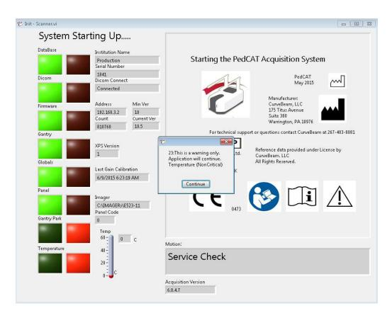
If one of more of these functions illuminates bright red, and remains bright red, it indicates a failure, please contact CurveBeam Technical Support if a light REMAINS on as follows:
